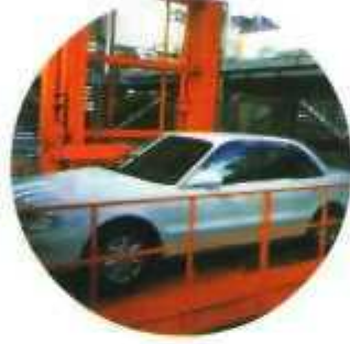
5. Through vertical and horizontal movement, send the vehicle to the nearest parking place.
